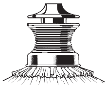
Correct position of the Mouthpiece on the Valve
