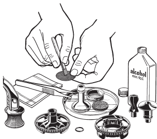
Manual cleaning with isopropyl alcohol (70 %) or detergent
